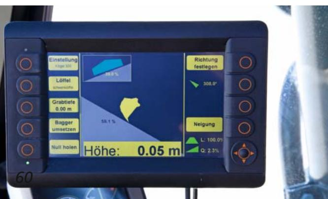
ifm's dialogue module (CR1082) serves as the display and data entry. Furthermore, the integrated PLC calculates the height.
