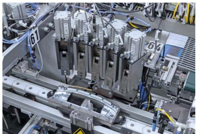
Fully automatic assembly of a vacuum cleaner nozzle at several stations.
