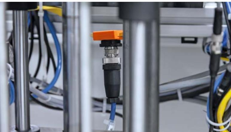
Sensors can be connected to any spot of the AS-i cable via a flat cable insulation displacement connector.
