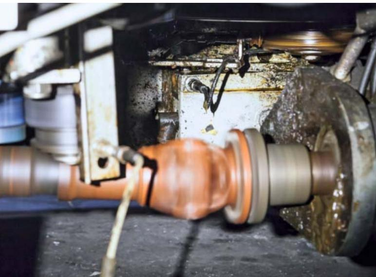
*Sensors allow vibration diagnostics in places that you could never access during operation for safety reasons.*
