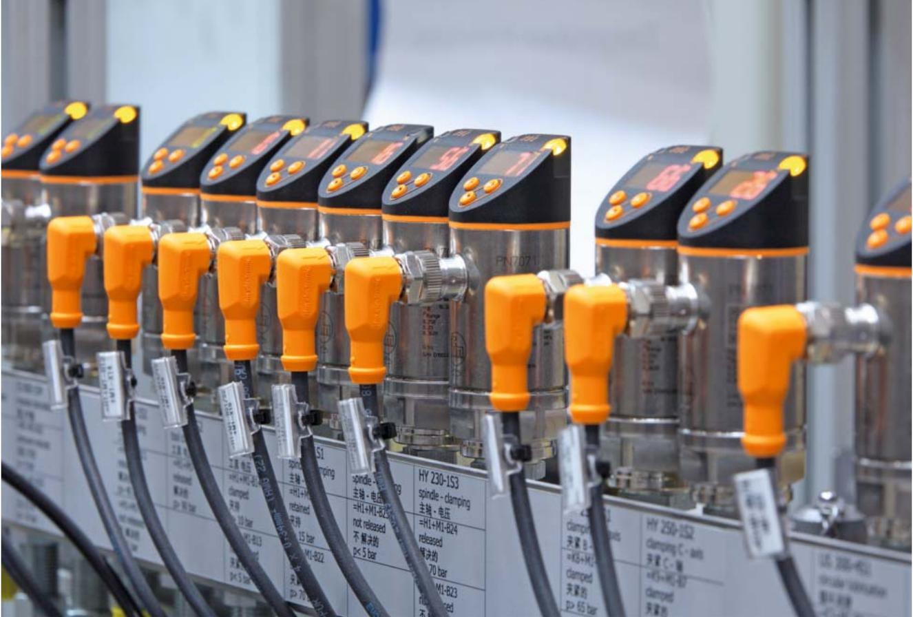
The numerous IO-Link sensors enable centralised parameter setting.
