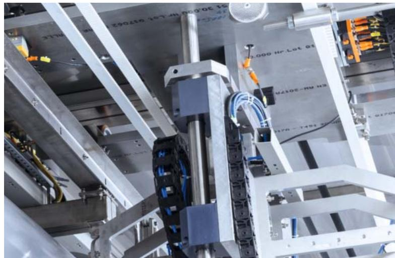
All sensors are connected to the bus system AS-Interface (AS-i) using modules.
