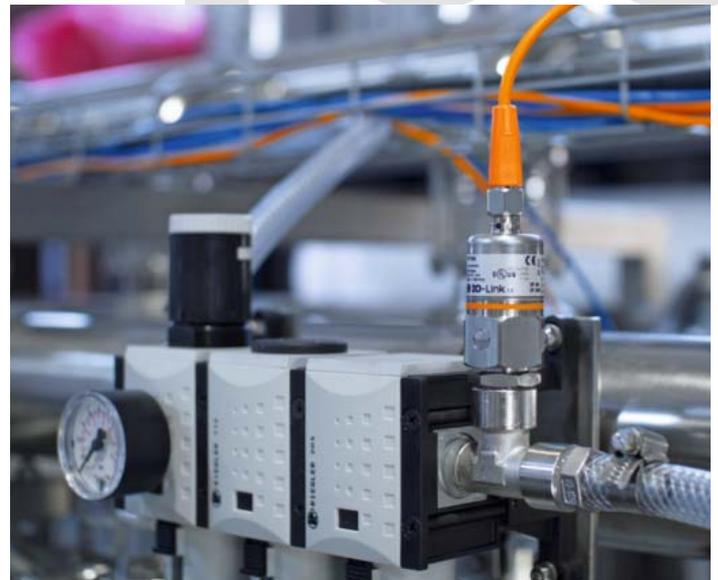
A pressure transmitter monitors the emptying process of the installation using compressed air
